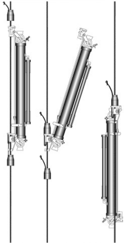
Nansen water bottles before (I), during (II), and after (III) reversing. (From Dietrich et al. 1980)
