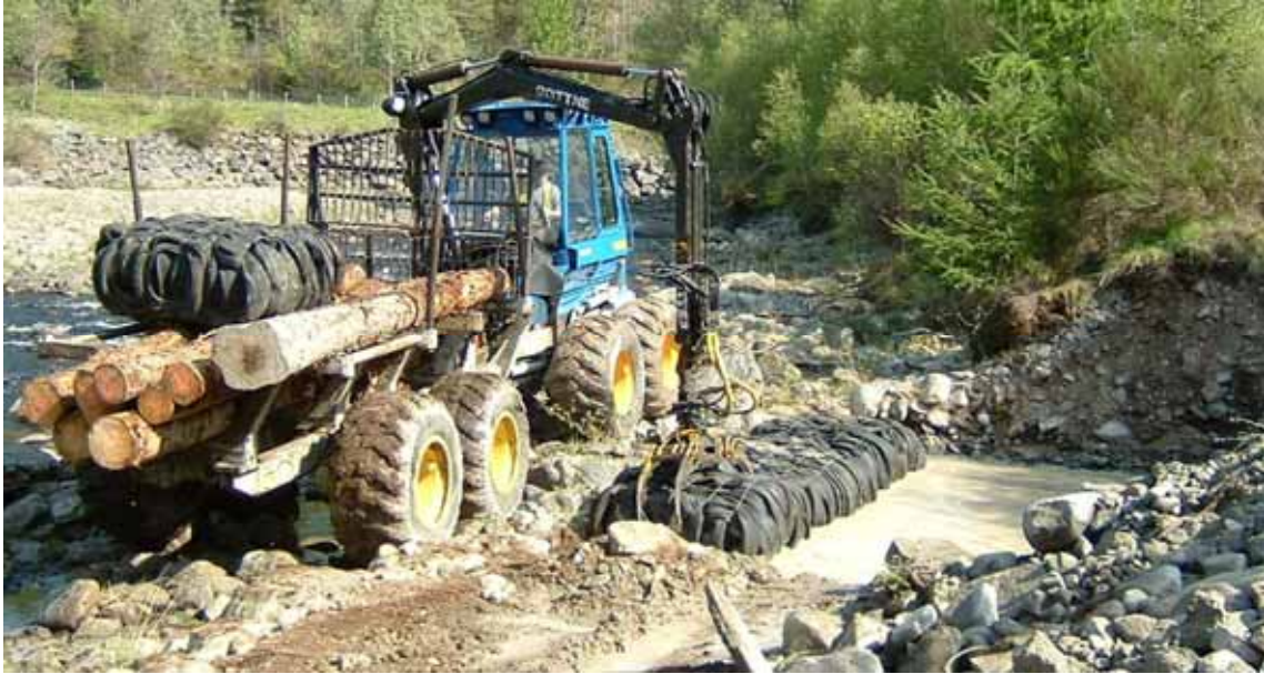
Figure 4.8 Forestry log transporter used at Glen Urquhart to access the site with tyre bales (courtesy Northern Tyre Recycling)
