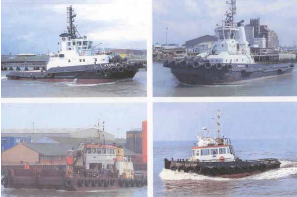
Figure 5.23 Tyres used as fenders on tugs and workboats (courtesy Sorrell Flood Protection)
