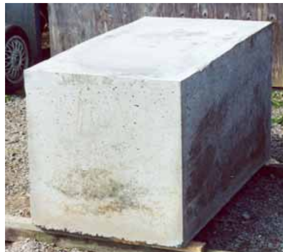
Figure 5.41 The tyre bale/concrete block product (courtesy Northern Tyre Recycling)
