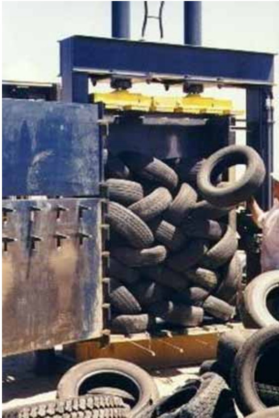
Figure 4.1 Loading baler hopper
