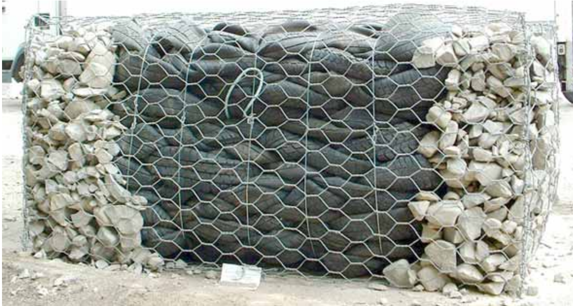
Figure 5.38 Tyre bale as centre fill for gabion box (courtesy Northern Tyre Recycling)
