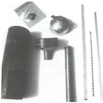
The traditional instruments for measuring snow consist of a precipitation gauge (outer can, funnel and inner measuring tube), a measuring stick, ruler, warm water to melt snow, and a metal sheet or clipboard to help extract snow cores.
