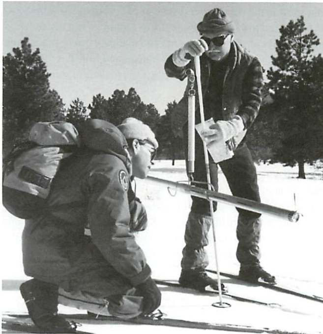
Special tubes for extracting snow cores and scales for weighing these samples greatly simplify the measurement of snow water content in snowy areas.
