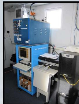
**Figure 3:** The NOAA GMD CATS in-situ GC with electron capture detection.
