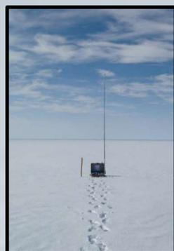
**Figure 1:** An example of NOAA air sampling, using a case holding two flasks which are pressurized with air. A long rod holds the collection tubing above ground.
