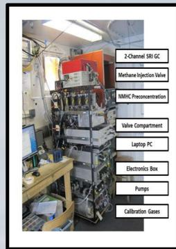
**Figure 2:** The INSTAAR in-situ GC instrument and sampling inlet inside TAWO at GEOSummit.
