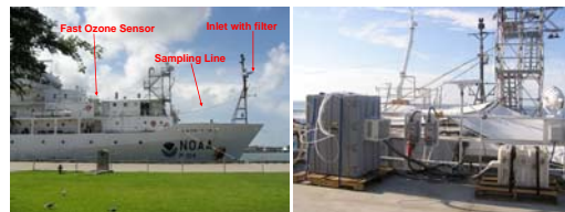
Figure 3. Configuration of the experiment during TexAQS 2006. Left: the inlet is located with a particle filter near the sonic anemometer, and the sampling line runs from the foremast to the sensor. Right: The fast ozone instrument was deployed on the third deck. The gray box contains the sensors, and the white box the pump system.
