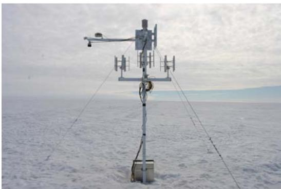
**Fig 1.** Distributed wireless sensor network observation platform
