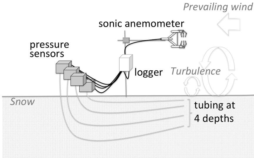
**Fig 1.** Schematic of experiment setup showing a sonic anemometer pointing into the prevailing wind and tubing for pressure sensors positioned in the snow below the sonic transducers.
