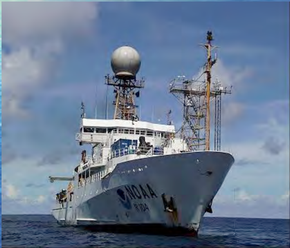
NOAA research vessel Ronald H. Brown at sea. Scientists mount instruments onto the bow tower to measure ozone fluxes over the oceans.
