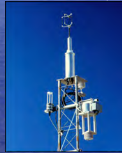
The bundle of instruments, from the top down: an anemometer/thermometer to measure wind speed and air temperature; in the cylinder below it a motion sensor that tracks how the ship is moving; a probe to sense mean air temperature and humidity; a e sensor of carbon dioxide and water; and a hygrometer to record the amount of water vapor in the air.
