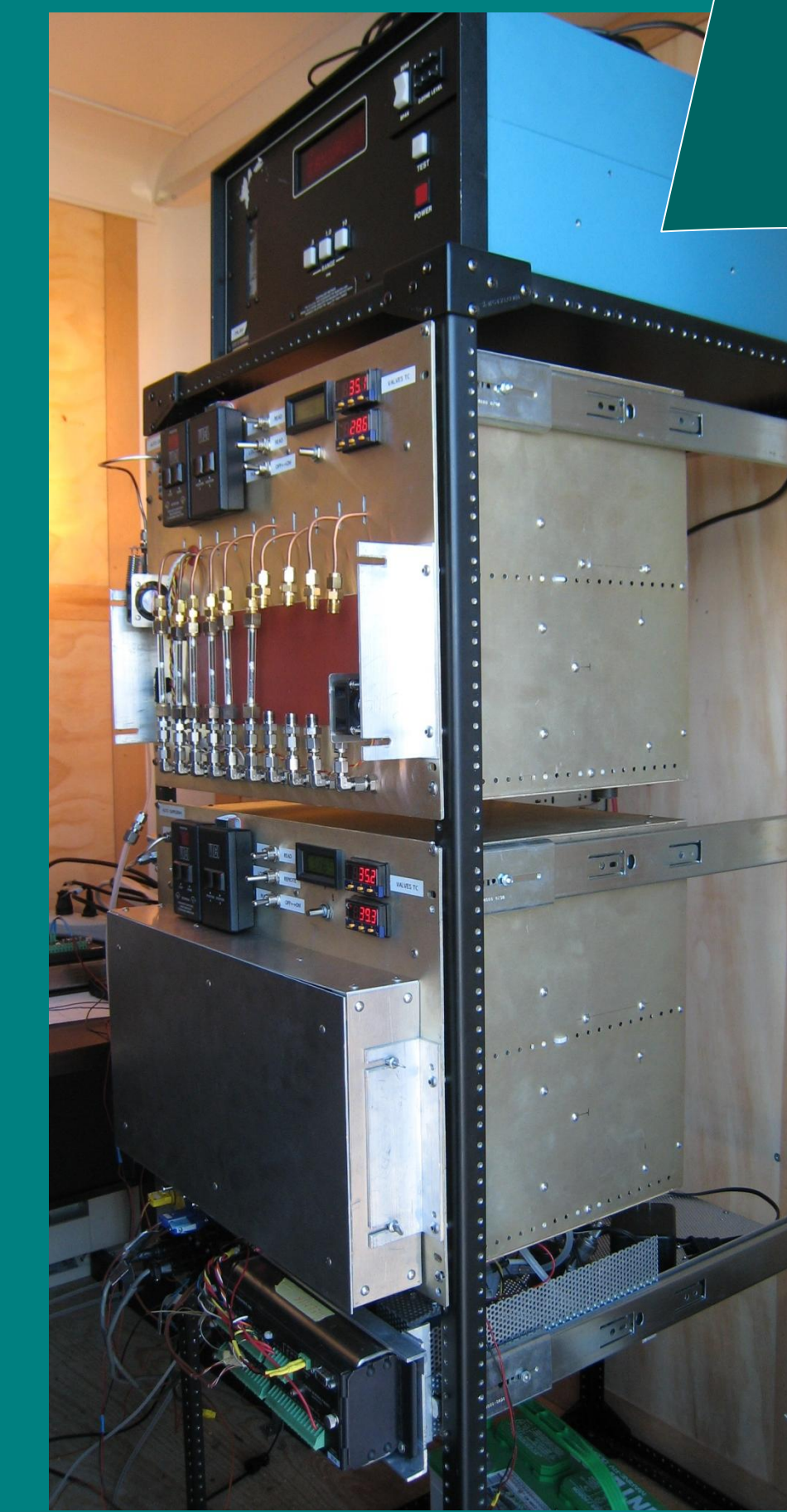
Inside the trailer that houses our instruments is this sampler, used to measure VOC emissions from tree leaves.
