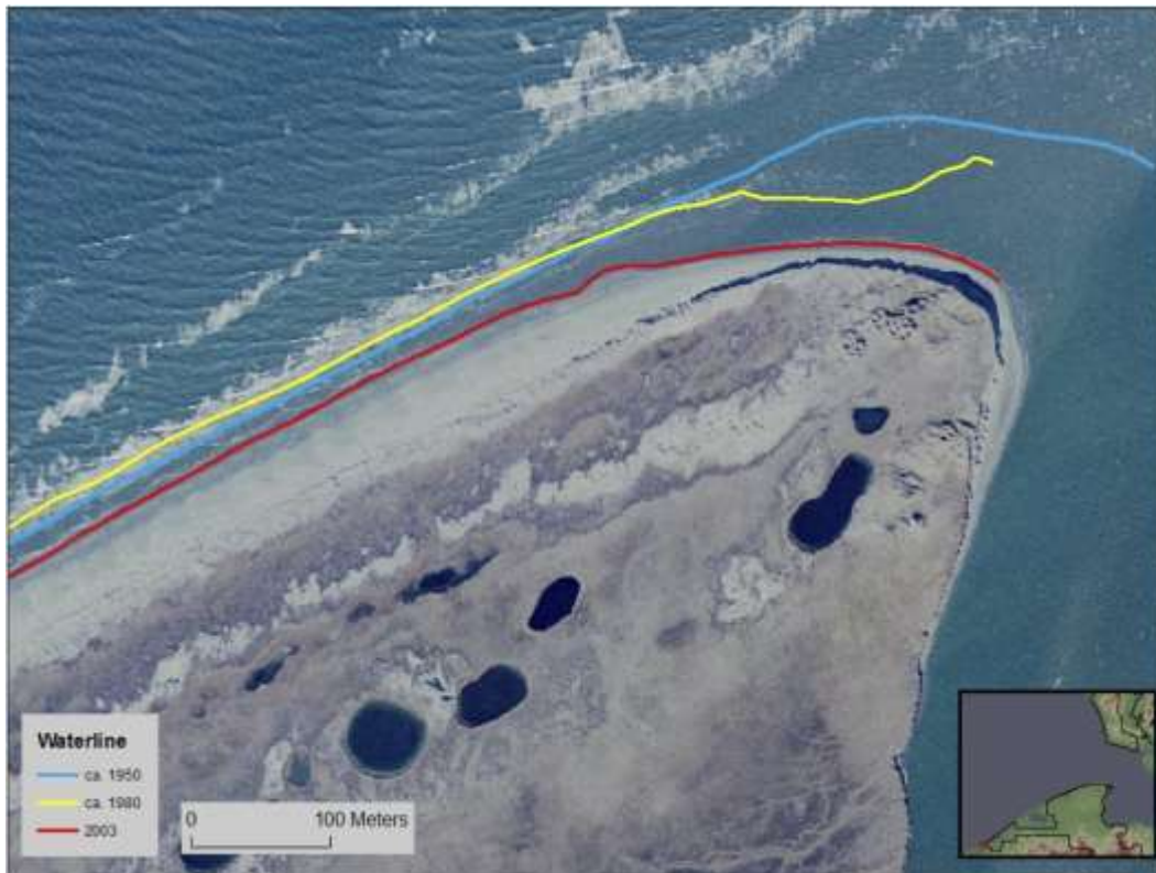
Figure 7. Map showing digital shorelines from the 1950, 1985, and 2003 superimposed on imagery from 2003, documenting tens of meters of bluff erosion. Data from Manley et al. (2007c, 2010).
