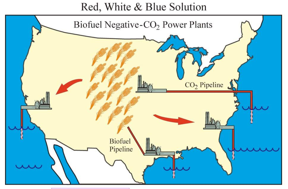
Cellulos ic Biofuels Electrical Power Generation Fail-Safe CO<sub>2</sub> Sequestration in Deep-Sea Sediments
