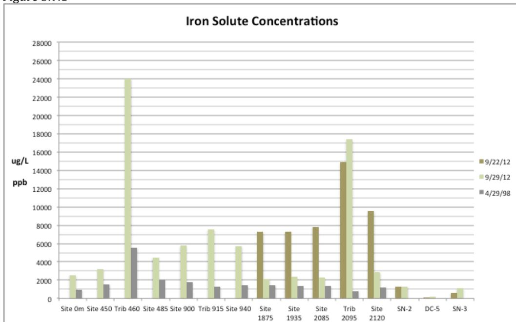
Iron is a difficult metal to evaluate against CDPHE Aquatic Life Standards due to its influence on water hardness and how it is calculated. But using the average water hardness value of 41 mg/L for the upper Snake River(Boyer et al, 1999) it is still possible to make a basic comparison that for most of the reach concentrations of iron exceeded the 1000ppb (ug/L) standard. However, as similarly observed with aluminum, the solubility of iron is particularly influenced by low pH.
