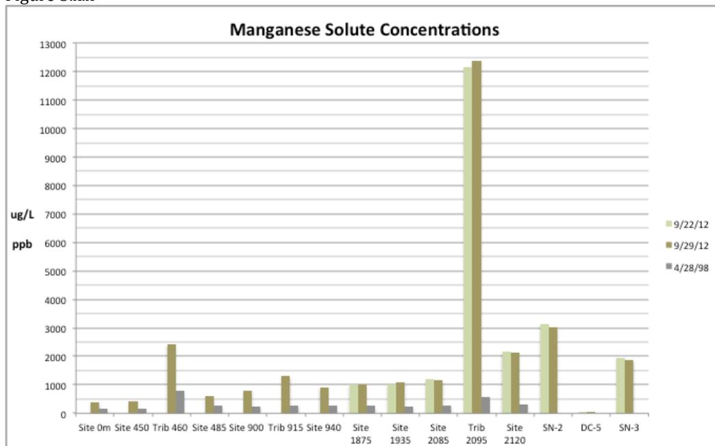
Manganese is difficult to evaluate against CDPHE Aquatic Life Standards due to its abundance as a mineral and taking into account how water hardness affects toxicity levels. By using water hardness value of 41 mg/L for the upper Snake River (Boyer et al, 1999) the acute to toxicity standard of manganese is 1556 ug/L. These levels are exceeded in the below Trib 2095 and remain so after the confluence with Deer Creek, though only slightly.
