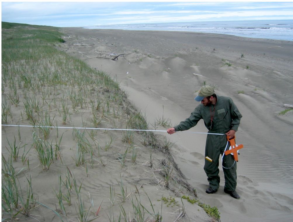
Figure 8. Photograph from 2006 showing field measurement of the distance of a low, eroding bluff from a benchmark, at the seaward side of a barrier island in BELA. This is one of many coastal monitoring stations established for BELA and CAKR (Jordan et al., 1999, 2008).
