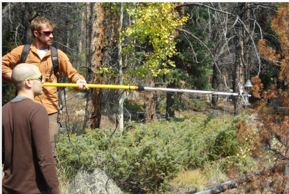
Ben Livneh and Dominik Schneider make albedo measurements with an albedometer (Courtesy Ben Livneh)
